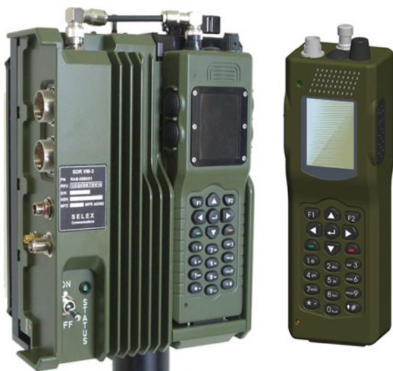
Fig. 13 Hand held soldier SDR and its vehicular adapter
